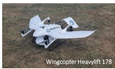
Speed: 150km/h max, 90km/h cruise Maximum take off weight: 16kg Flight time: Up to 120 minutes Wind Resistance: Up to 15m/s Dimensions: 178cm x 132cm x 52cm Range: Up to 100km Payload Up to 6kg 1000s of BVLOS kilometres flown
