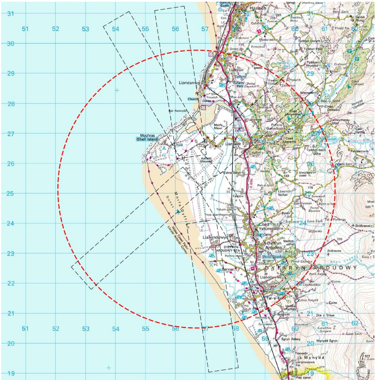
Figure 5 - The proposed Aerodrome Traffic Zone (red dashes) and Runway Protection Zones (black dashes, post aerodrome licencing) at Llanbedr superimposed on a 1:50,000 scale local map to show the full horizontal extent
