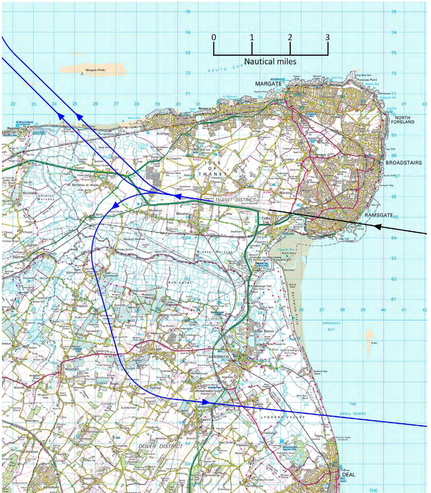
Figure 17 – Runway 28 Approach Procedures (1:50,000 Ordnance Survey Mapping) showing the MAP (go-around) tracks overland from a left or right turn at the end of the runway
