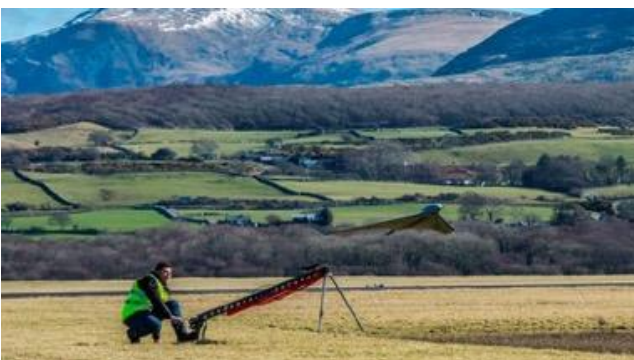
Fig. 3e – C-Astral Bramor used to explore the potential for mapping and surveying drones
