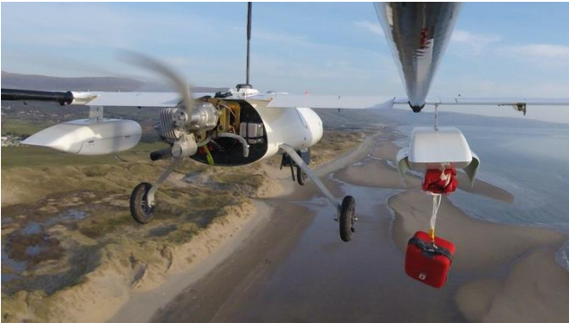
Fig. 3a – Penguin B used to explore the potential for aeromedical delivery drones
