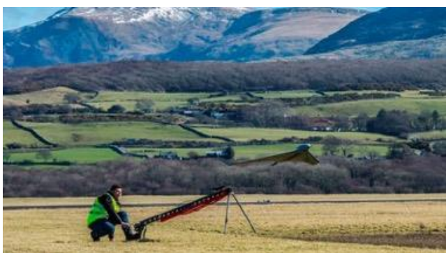
Fig. 2e – C-Astral Bramor used to explore the potential for mapping and surveying drones
