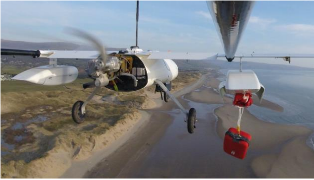
Fig. 3a – Penguin B drone used to explore the potential for aeromedical delivery
