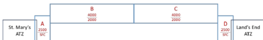
Figure 2 Temporary Danger Area Design (vertical layout)
