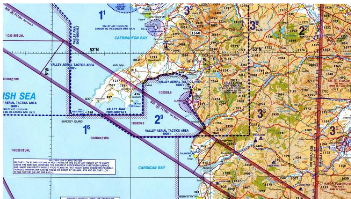
Figure 3 - UK aviation chart from 2002 showing the ATZ and Danger Area (D202) at and around Llanbedr Aerodrome prior to QinetiQ/MOD vacating the site in 2004
