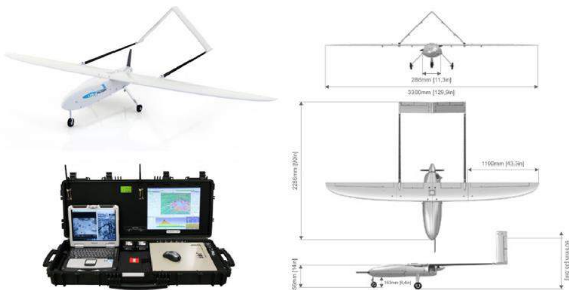
Figure 9 - the Penguin has a 3.3m wingspan, a 21.5kg maximum take-off weight, a dash speed of 36 \text{ ms}^{-1} (70 knots) and is powered by a 28cc, 2.5hp two-stroke, single-cylinder petrol engine
