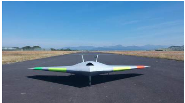
Fig. 2f – BAE Systems/University of Manchester MAGMA aerodynamics test drone
