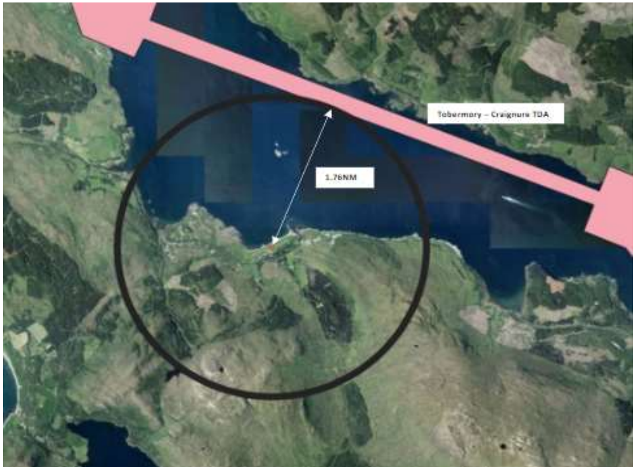
FIGURE 1: DISTANCE OF CONSTRAINED LEG IN TOBERMORY - CRAIGNURE TDA RELATIVE TO CENTRELINE OF GLENFORSA AIRFIELD
