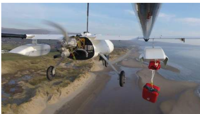
Fig. 2a – Penguin B used to explore the potential for aeromedical delivery drones
