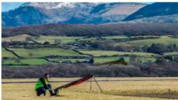
Fig. 3e – C-Astral Bramor used to explore the potential for mapping and surveying drones
