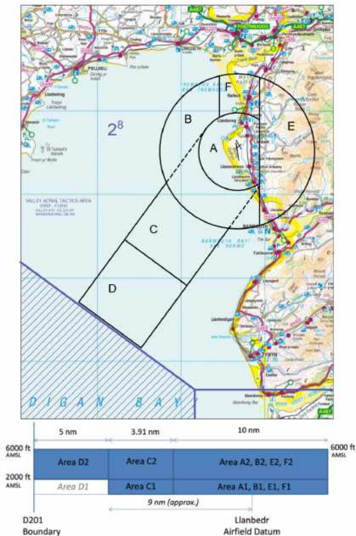
Fig. 1 - Final Airspace Design (Option #2b) for ACP-2019-58, Llanbedr Danger Area, incorporating the revisions suggested from the consultation
