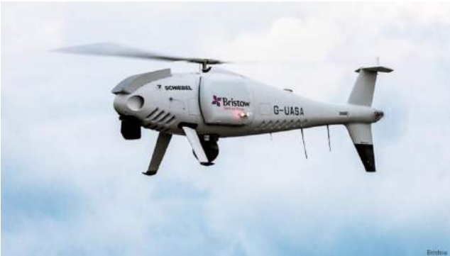
Fig. 4c – Scheibel S100 Camcopter used to explore the potential for search/rescue drones
