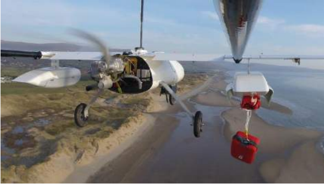
Fig. 4a – Penguin B used to explore the potential for aeromedical delivery drones
