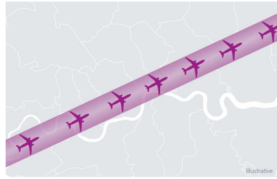
A narrow flight corridor using accurate satellite navigation (PBN)
