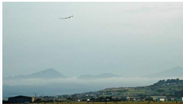
Figure 5d – Astigan solar-powered high altitude, long endurance (HALE) vehicle
