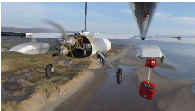
Figure 5a – Penguin B used to explore the potential for aeromedical delivery drones
