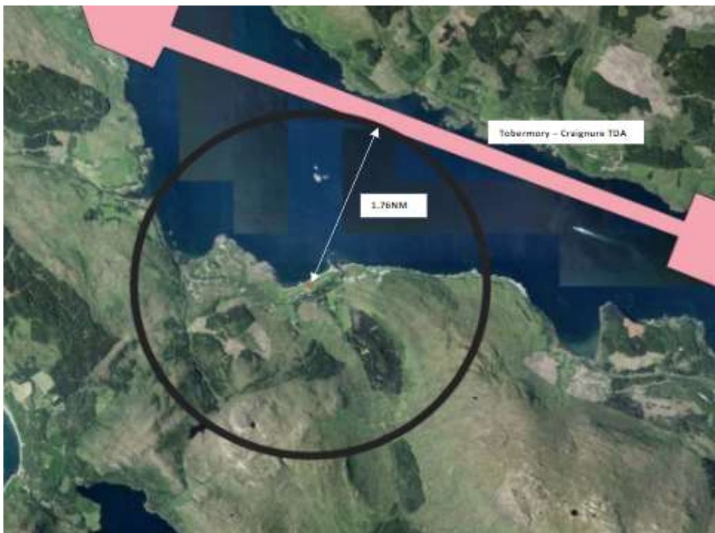
FIGURE 8: DISTANCE OF CONSTRAINED LEG IN TOBERMORY - CRAIGNURE TDA RELATIVE TO CENTRELINE OF GLENFORSA AIRFIELD
