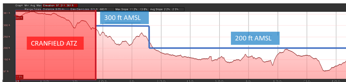
Figure 3: NBEC flight path elevation and assumed ground heights
