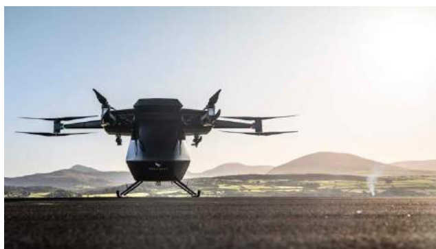
Fig. 2b – Vertical Aerospace electric Urban Air Mobility (UAM) vehicle
