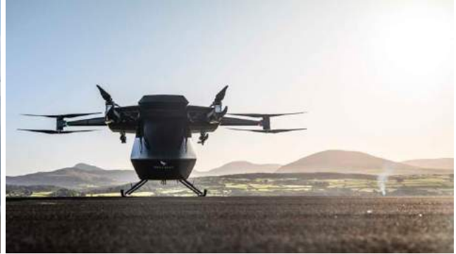
Figure 5b – Vertical Aerospace electric Urban Air Mobility (UAM) vehicle
