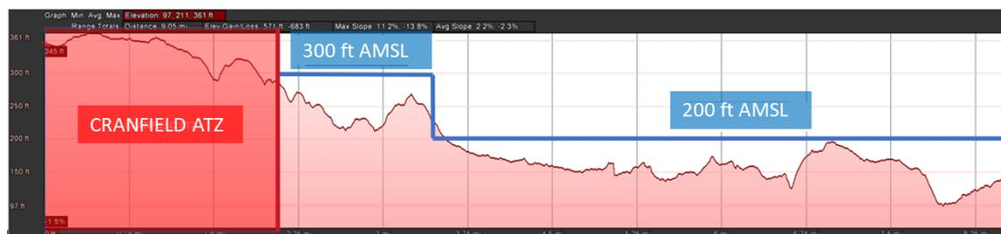
Figure 5: NBEC flight path elevation and assumed ground heights
