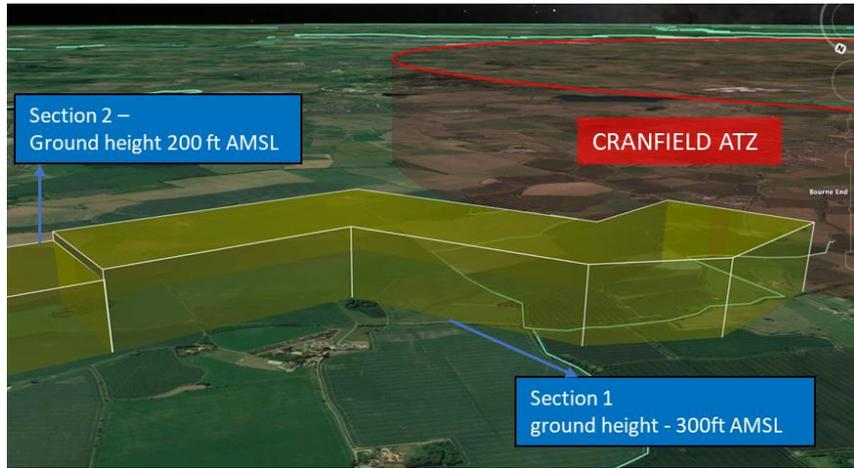
**Figure 6: NBEC flight path Sections – assumed ground heights**
