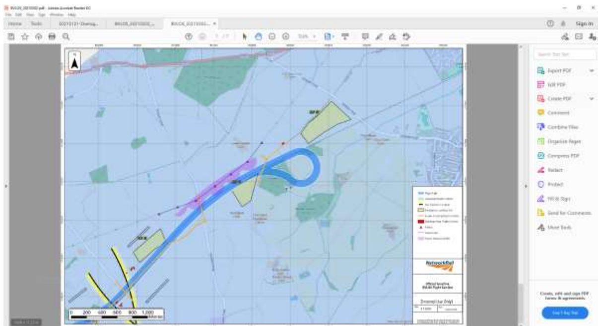
Figure 6 - ESRO ARC GIS Map, detailing proposed aircraft track in relation to East to West Railway Line, including GO/NO GO boundaries, alternate landing sites, higher risk urban areas, proximity to power lines
