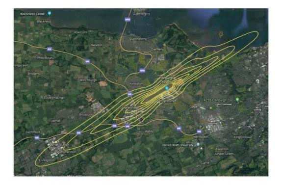
Map B: 2018 LAeq Summertime contour overlaid on the mean departure and arrival flight paths using EDI radar data supplied via ERCD
