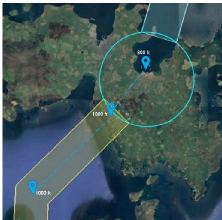
Figure 11 Return route followed by the aircraft in case of C2 failure in TDA-A.
