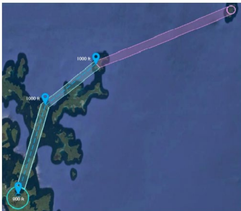
Figure 12 Return route followed by the aircraft in case of C2 failure in TDA-B and TDA-C.
