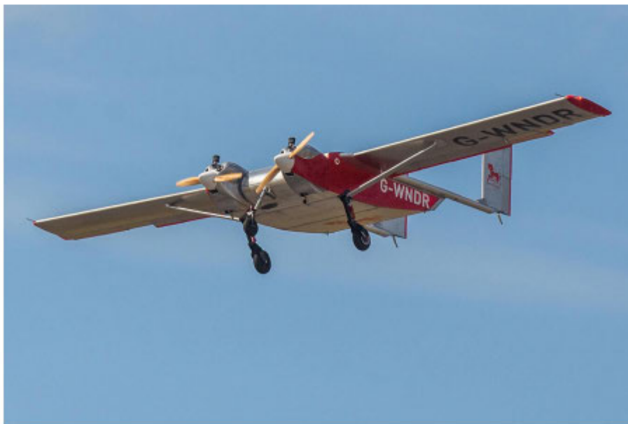
Figure 1 ULTRA UAS has a 10 m wingspan and cruises at 75 knots
