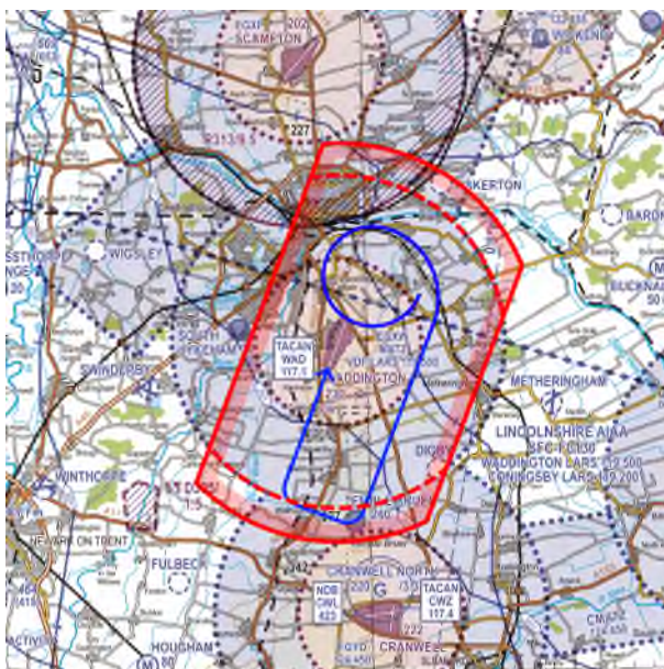
Figure 12 - RW02 Automatic Landing Profile for a Descent to Final Approach
