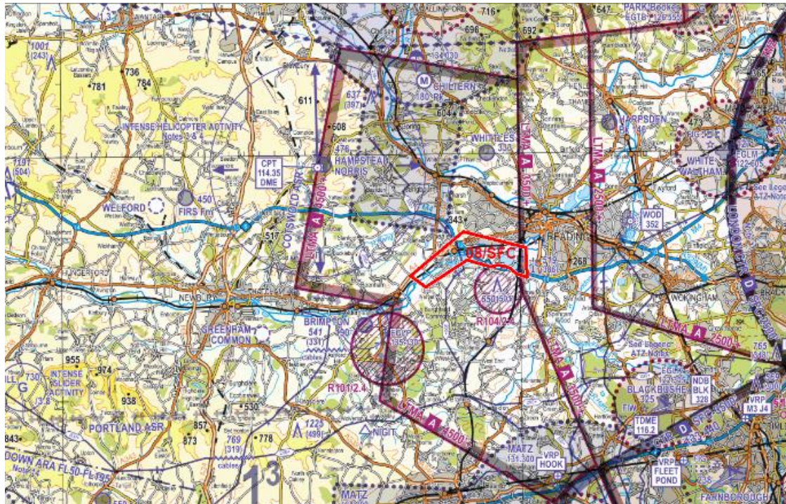
Figure 6 Proposed Final TDA Shape at SFC-800ft AMSL Following Feedback ON CAA 1:250K England South Chart
