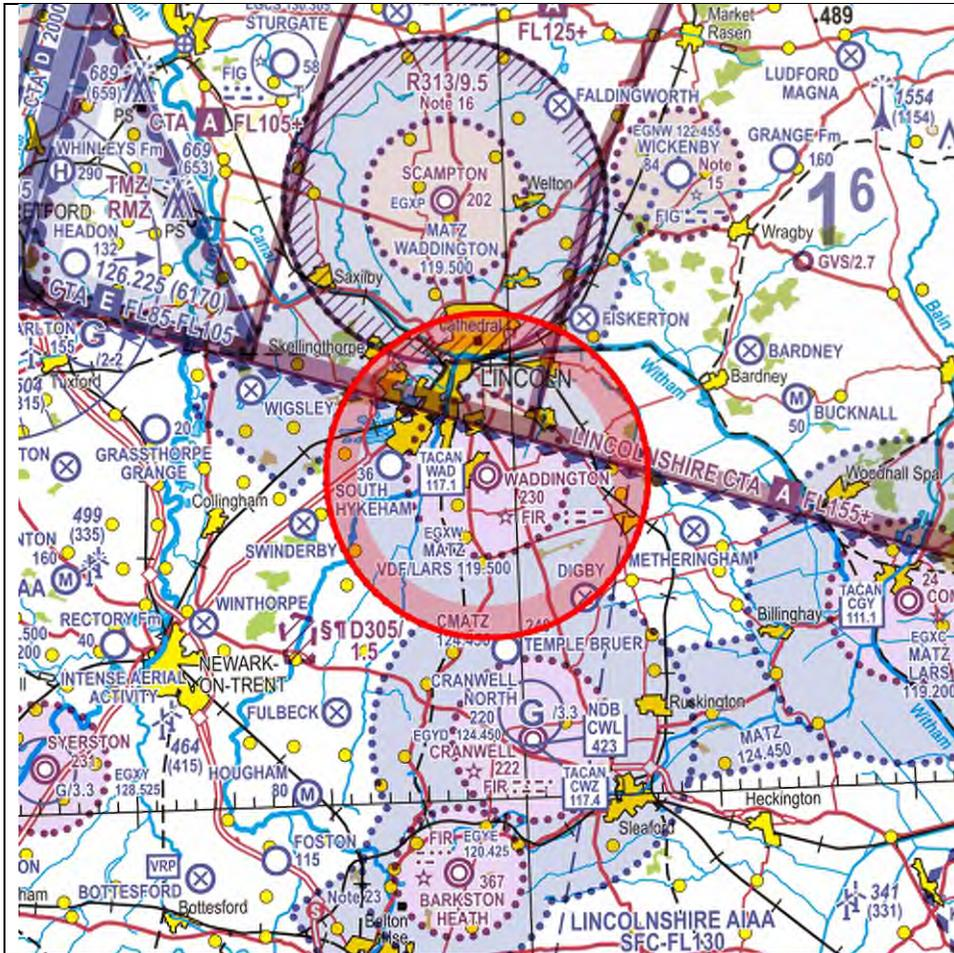
**Lateral Dimension:** 5 nm radius circle centred on RAF Waddington's aerodrome reference point<sup>1</sup> (ARP).
