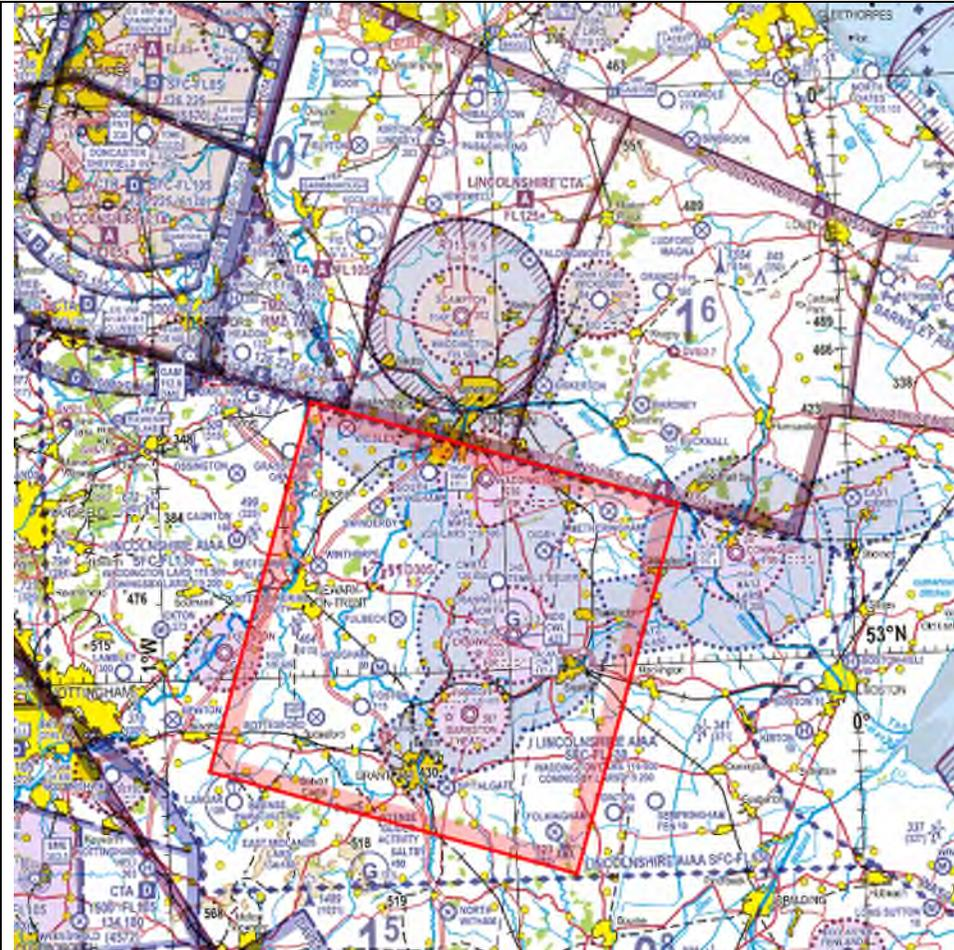
**Lateral Dimension:** 20 x 20 nm rectangle aligned to and abutting the southern edge of the Lincs CTA.
