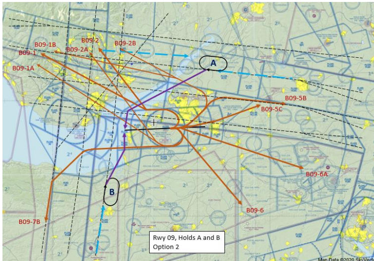
Figure 32: Runway 09 Option 2 with Holds A and B
