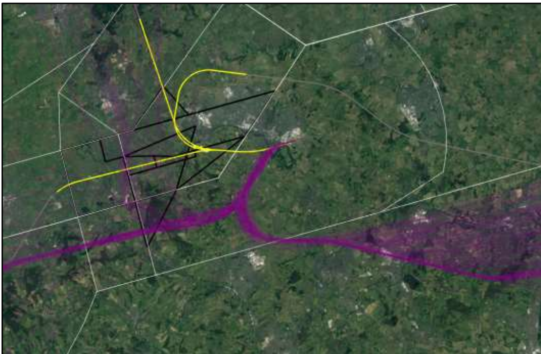
Figure 34: Existing departure swaths (purple) and W SID Group 8 Period 1 illustrative centrelines (yellow) from Luton's westerly runway
