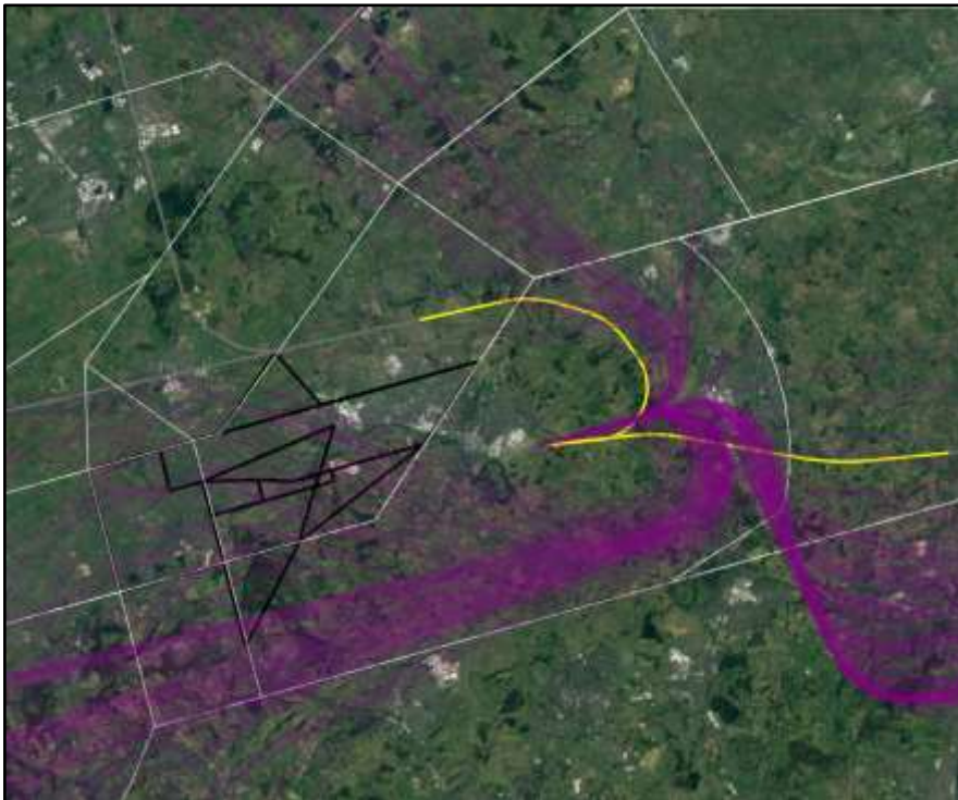
Figure 41: Existing departure swaths (purple) and the E SID Group 6 Period 2 illustrative centrelines (yellow) from Luton's Easterly runway
