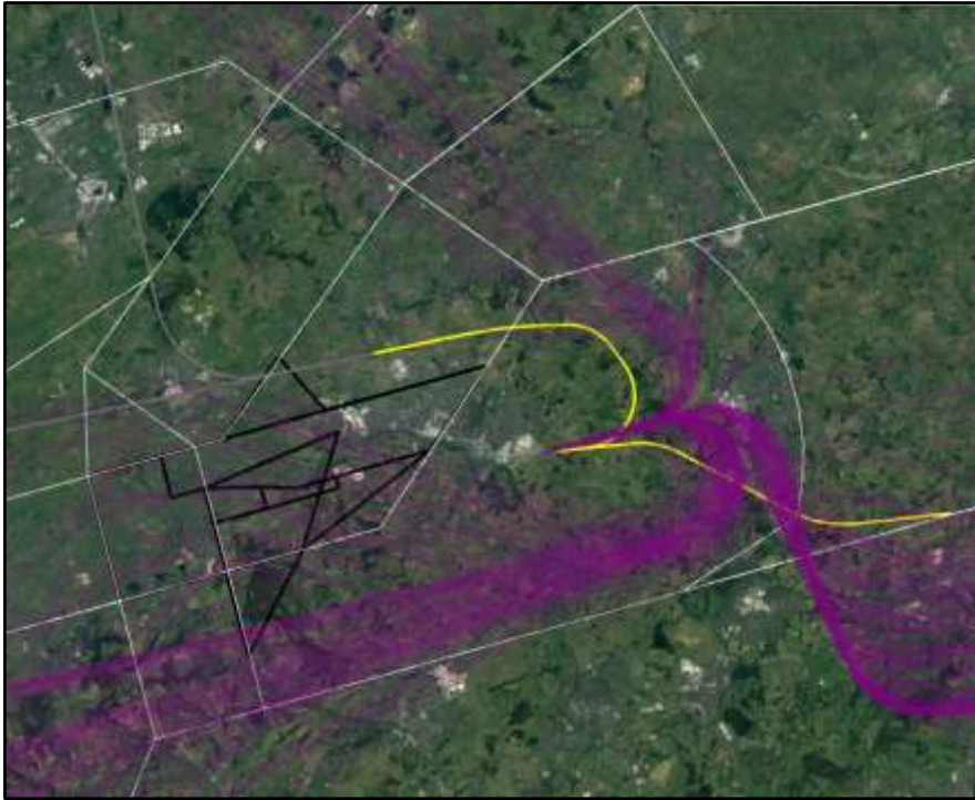
Figure 40: Existing departure swaths (purple) and the E SID Group 6 Period 1 illustrative centrelines (yellow) from Luton's Easterly runway
