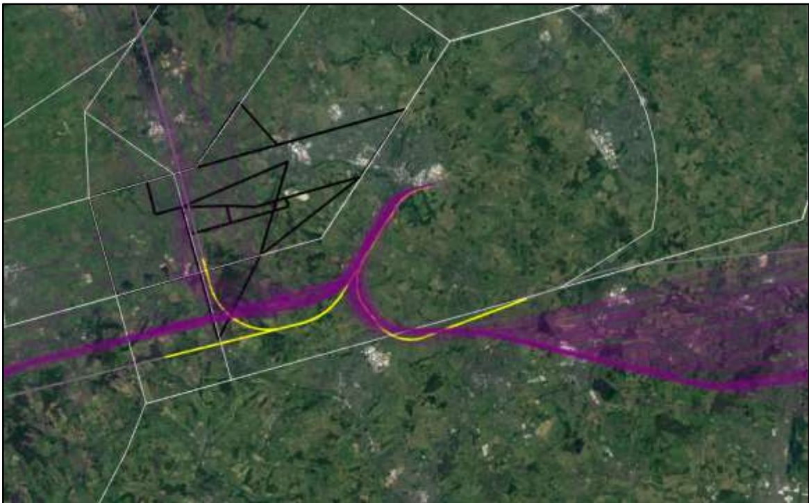
Figure 30: Existing departure swaths (purple) and W SID Group 6 Period 2 illustrative centrelines (yellow) from Luton's westerly runway
