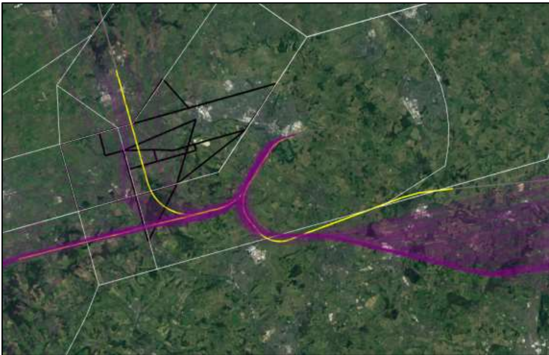
Figure 27: Existing departure swaths (purple) and W SID Group 4 Period 2 illustrative centrelines (yellow) from Luton's westerly runway
