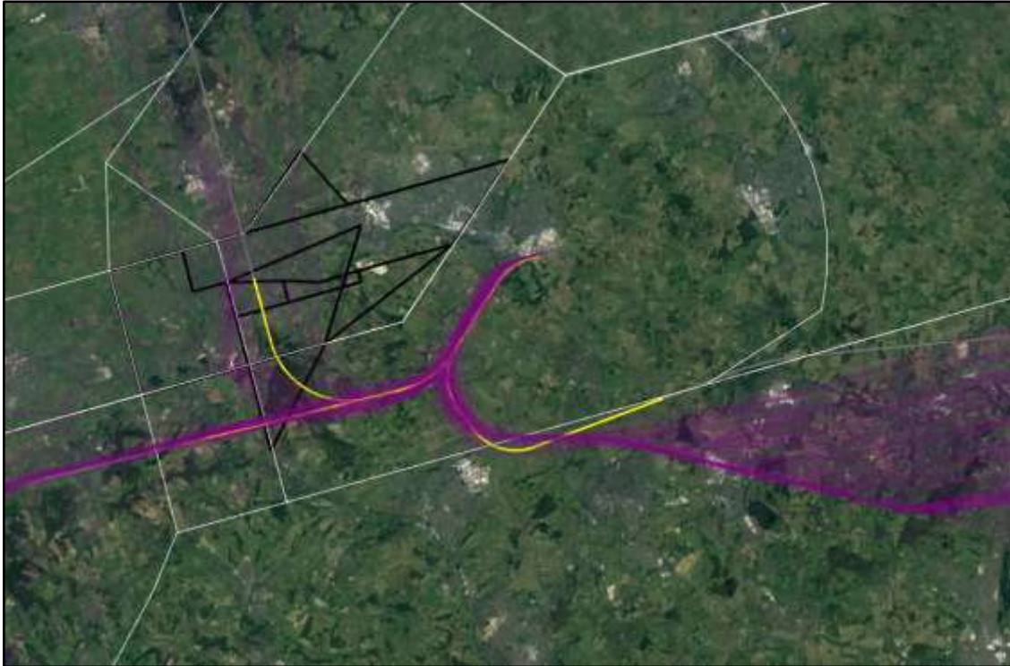
Figure 31: Existing departure swaths (purple) and W SID Group 7 Period 1 illustrative centrelines (yellow) from Luton's westerly runway
