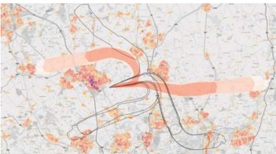
Figure 24 Easterly SID Group 5 overflight (centreline), with population density and baseline (black outline).
