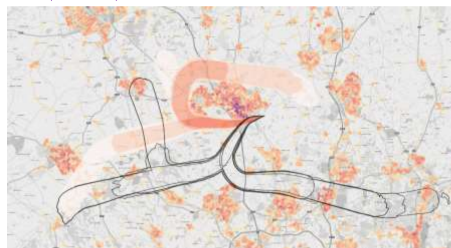
Figure 16 Westerly SID Group 8 overflight night (centreline), with population density and baseline (black outline).
