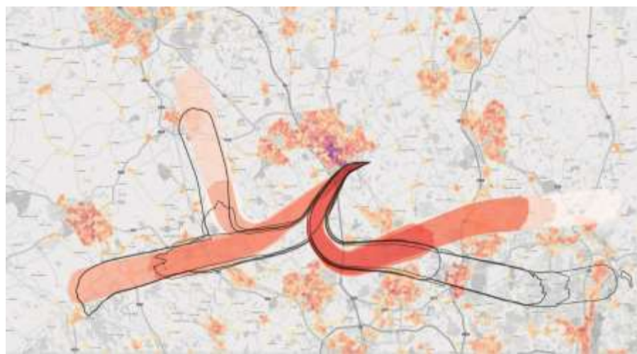
Figure 11 Westerly SID Group 5 overflight (centreline), with population density and baseline (black outline).
