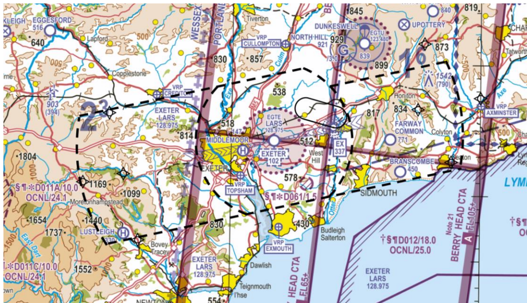
Figure 18 – 6x5 Lozenge and IF-Protected Expanded Zone Avoiding Dunkeswell
