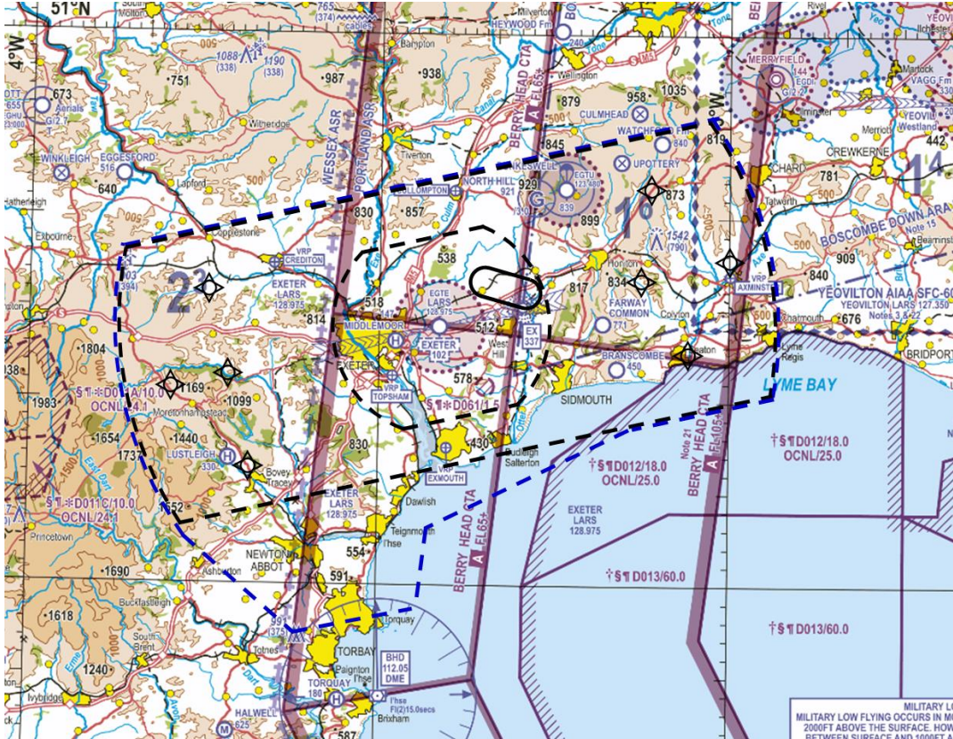
Figure 25 – 6x5 Lozenge and IAF-Protected Expanded Zone plus Upper Zone to the South
