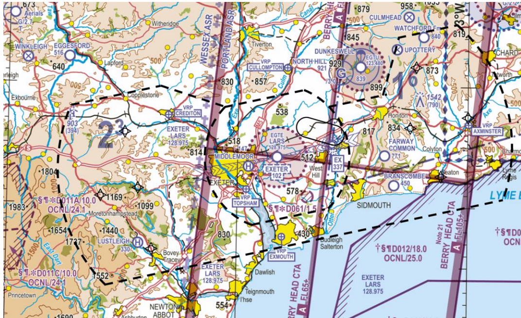
Figure 20 – 6x5 Lozenge and IAF-Protected Expanded Zone Avoiding Dunkeswell
