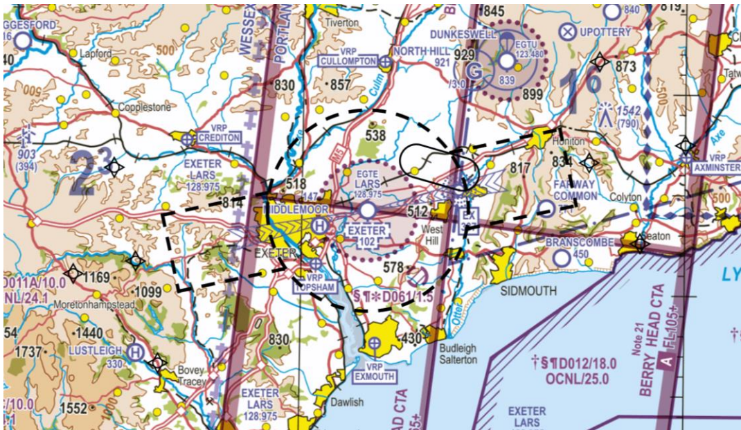
Figure 14 – 5 nm Circle with 4 nm Wide Stubs
