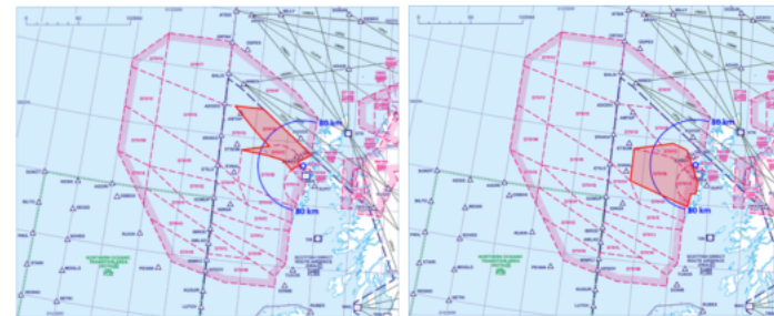
Figure 2: Sounding Rocket 80km Safety Range – Diagram Depicting Two Potential Options for D701 Activation
