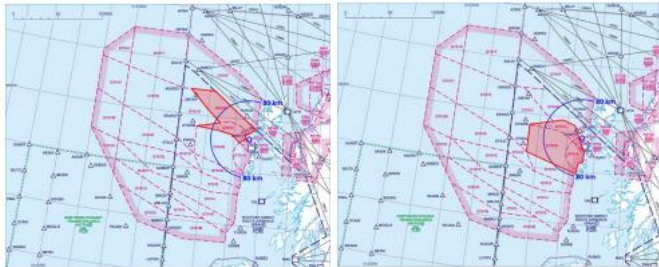
Figure 3: Sounding Rocket 80km Safety Range – Diagram Depicting Two Potential Options for D701 Activation
