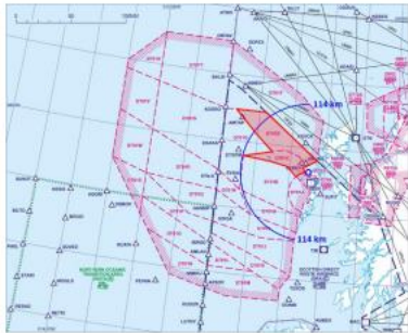
Figure 4: Sounding Rocket 114km Safety Range – Diagram Depicting Potential D701 Activation
