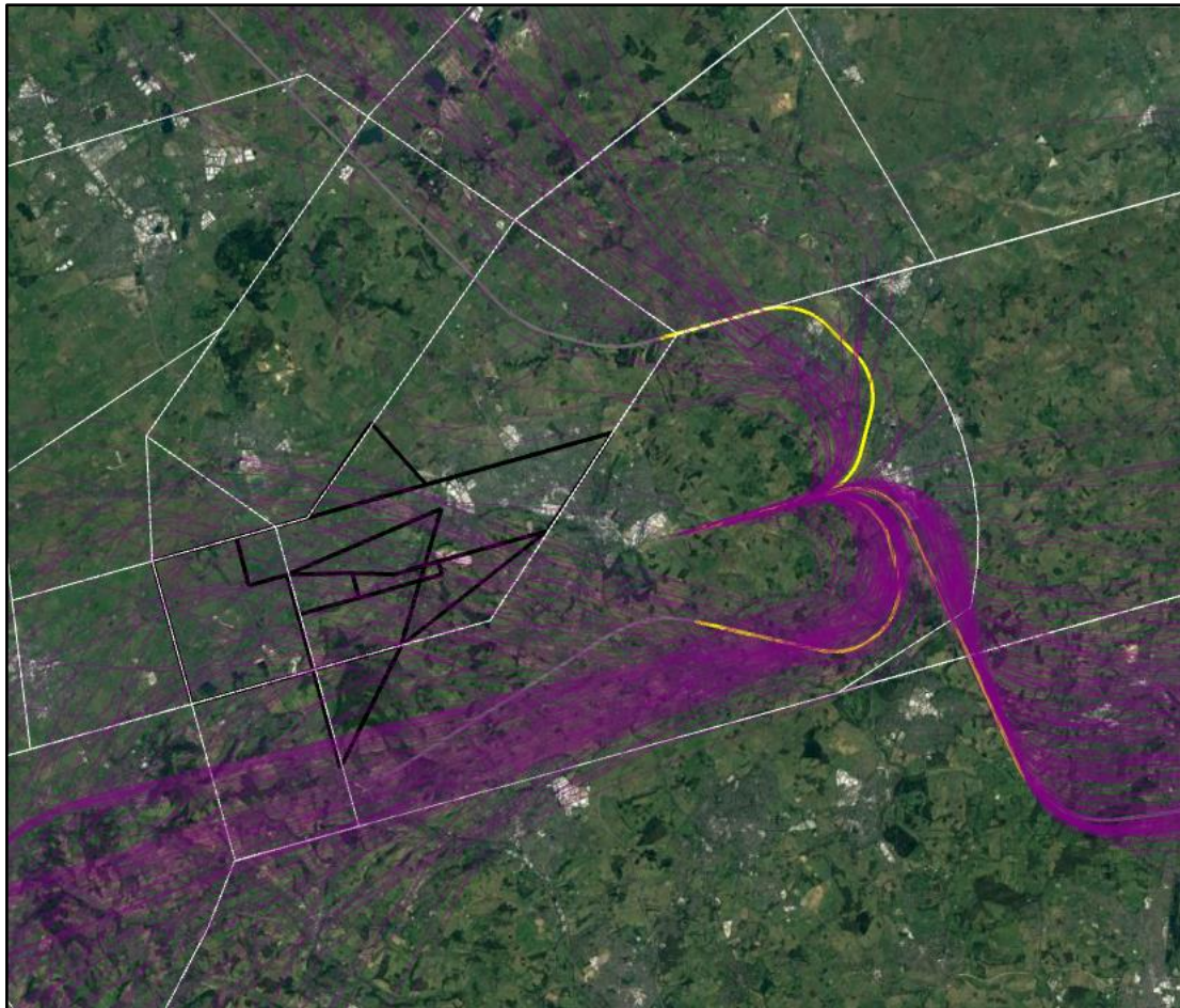
Figure 37: Existing departure swathes (purple) and the E SID Group 3 illustrative centrelines (yellow) from Luton's Easterly runway
