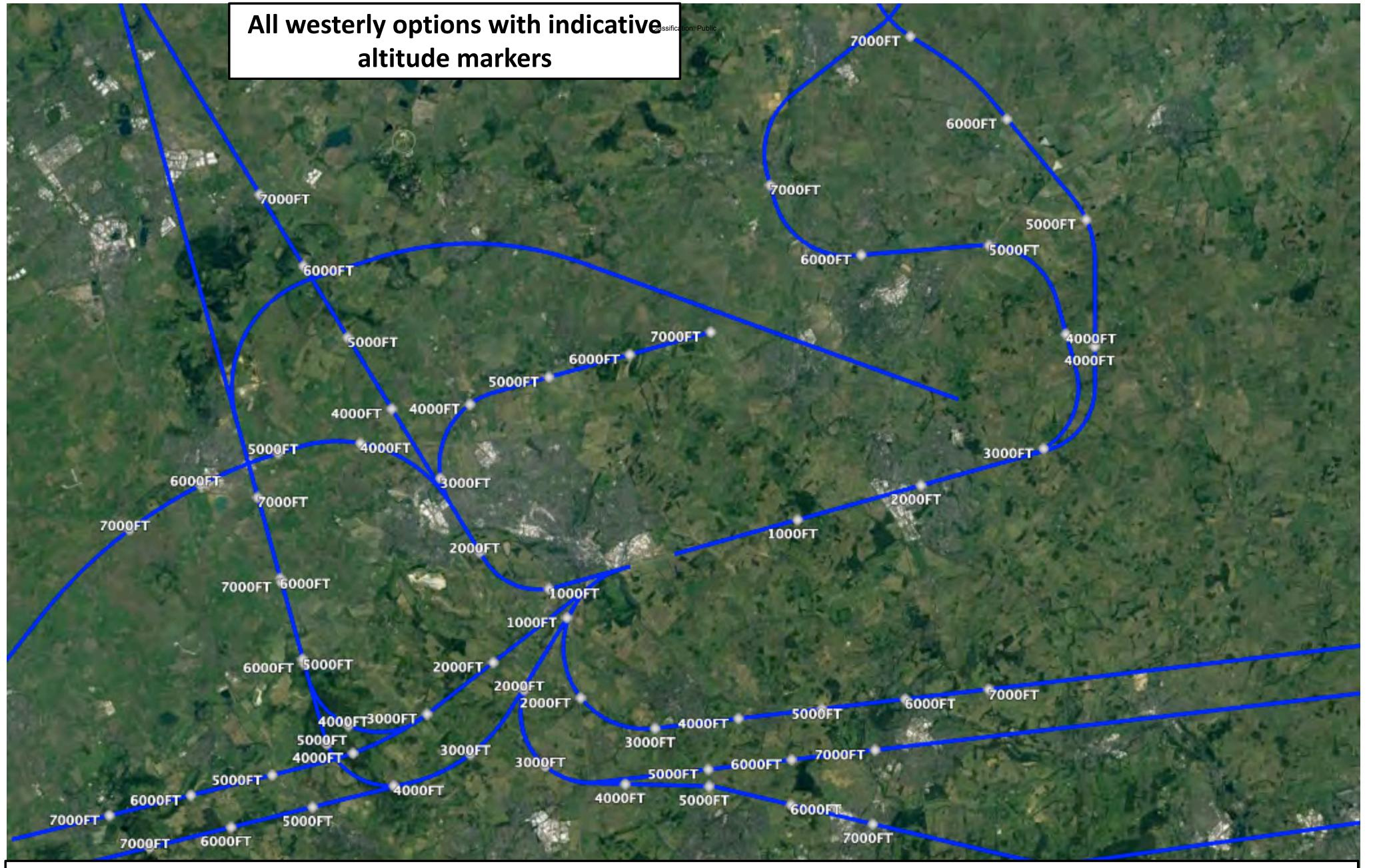
1,000ft altitude markers based on 8% climb gradient or 3° (5.24%) descent gradient. For departures, this assumes the aircraft starts climb from the very end of the runway. However, aircraft start climb approximately 2/3 down the runway so the altitudes shown here can be considered pessimistic.
