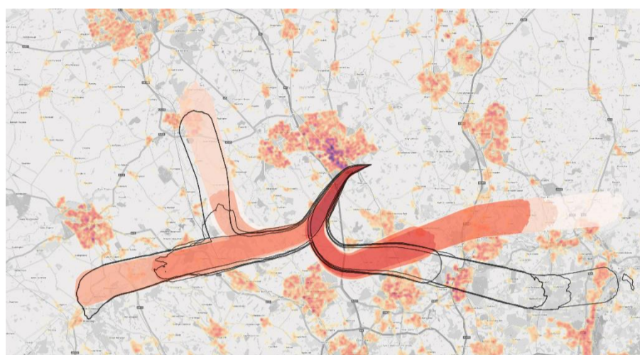
Figure 8 Westerly SID Group 2 overflight (centreline), with population density and baseline (black outline). Note this option would retain some vectoring which is not shown in these centreline contours.
