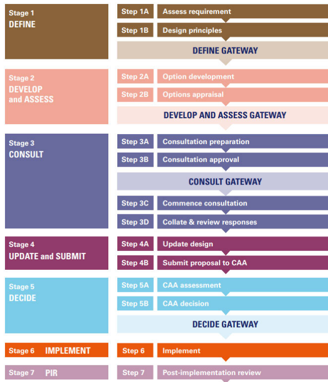
Figure 2 CAP 1616 High-level Process
