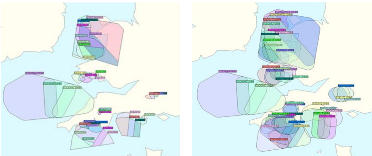
Figure 38 Airspace today (left) and Airspace with 10nm buffer applied to SUA (right)
