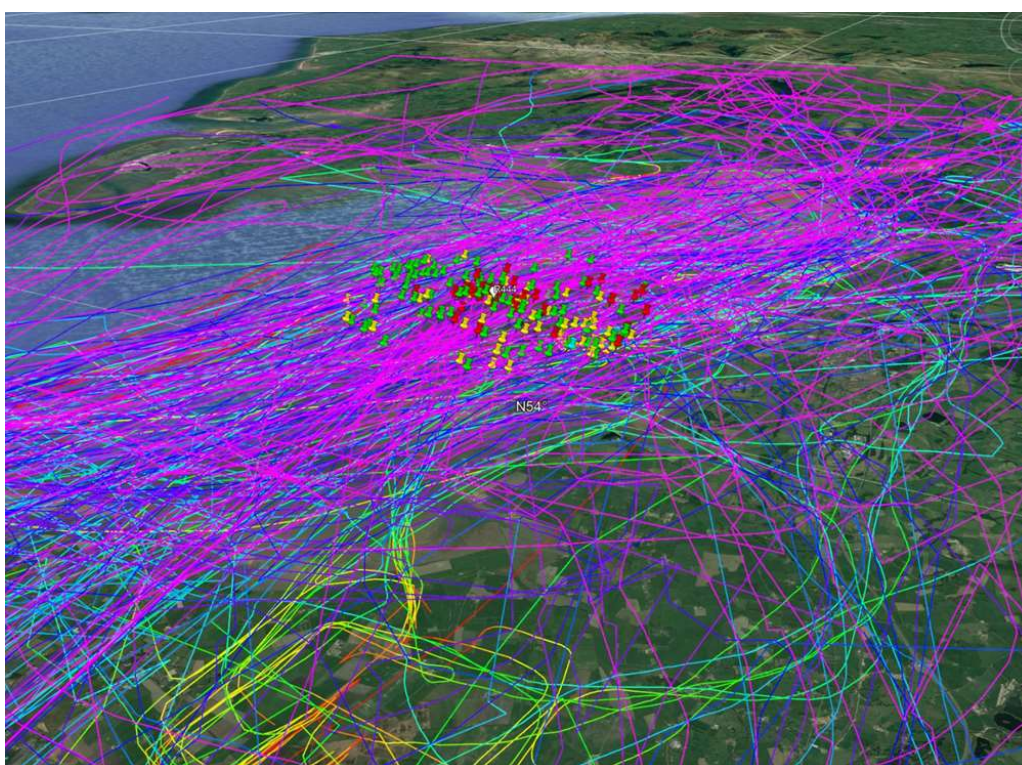
180 infringements of R444; track with rainbow altitudes (red: 0m to pink: 609m+) Pushpin defines point of closest proximity w.r.t horizontal and vertical distance Pushpin colour defines a/c type (red: microlight, green: plane, yellow: helicopter)
