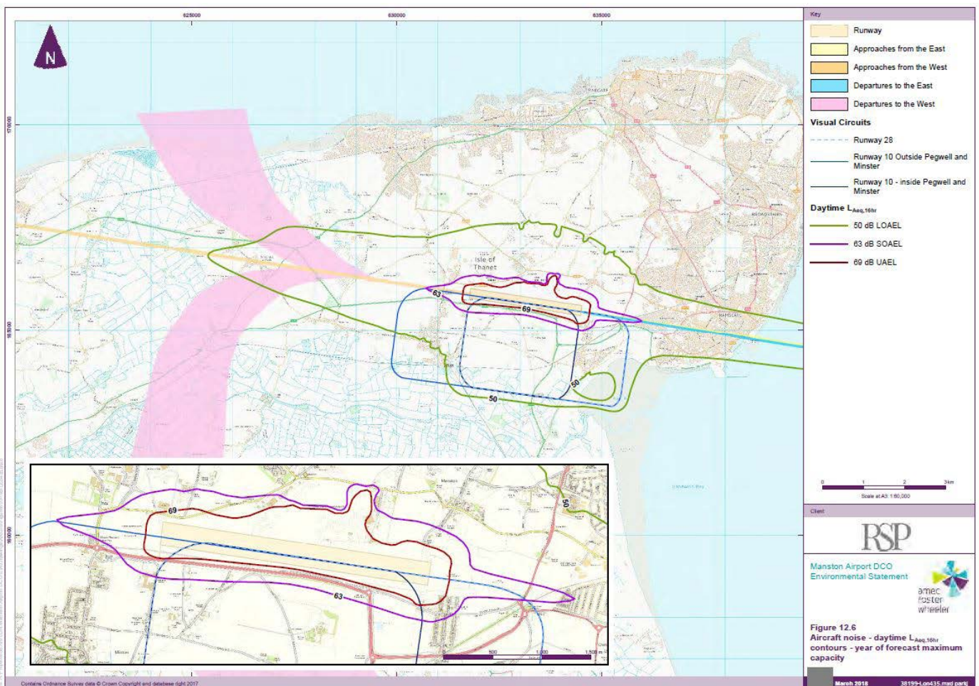
Figure 8 - DCO Environmental Statement Year of Maximum Forecast Capacity Daytime LAeq, 16hr Contours
