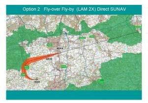
This option uses the same turn as described in Option 0, however, the track adjustment at KKE15 is removed and waypoint NEW 11 is placed on the course that aircraft would nominally roll out of the turn. WP NEW09 maintains the requirement for aircraft to be above 3200ft at a point abeam the original KKE09 and NEW 11 maintains the restriction of aircraft not climbing 4000ft at the point abeam KKE11. NEW11 lifts the speed restriction from 220 KIAS to 250 KIAS.
