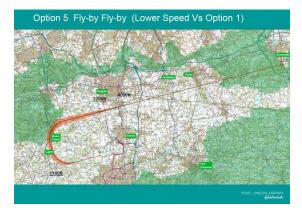
Option 5 uses the same methodology as option 1 which incorporates two 90° turns at fly-by waypoints followed by a direct track to SUNAV at 5000ft. The speed is reduced in the turn to 200 KIAS and this results in the waypoints being placed closer together, as a result the turn is completed to the south of that designed in Option 1. The 200 KIAS restriction is lifted to 250 KIAS at NEW12 creating a point of acceleration.
