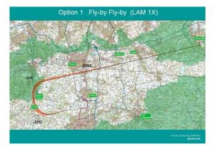
This was the previously published LAM 1X SID and was previously published in the UKAIP 2013. Aircraft fly straight ahead and make the first turn at KKW04 not below 2500ft. Two 90° turns at the fly-by waypoints KKW04 and KKN06 result in aircraft tracking 079° (True) following the turn. The turn is coded Track to Fix which results in a relatively small degree of dispersion in the turn. Aircraft must be below 4000ft at WP KKE14 where the speed restriction of 220 KIAS is raised to 250
