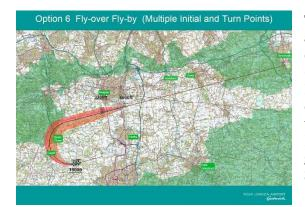
This option is an amalgam of Options 3 and 4 and is expected to result in a degree of track dispersion in, and following, the turn. Option 6 brings the paths to a common waypoint at KK11A and from there a concentrated track of traffic to SUNAV at 5000ft utilising a Track to Fix Path Terminator, unlike the Course to Fix used in Option 3 which leads to a more gradual concentrating of the tracks closer to SUNAV.
