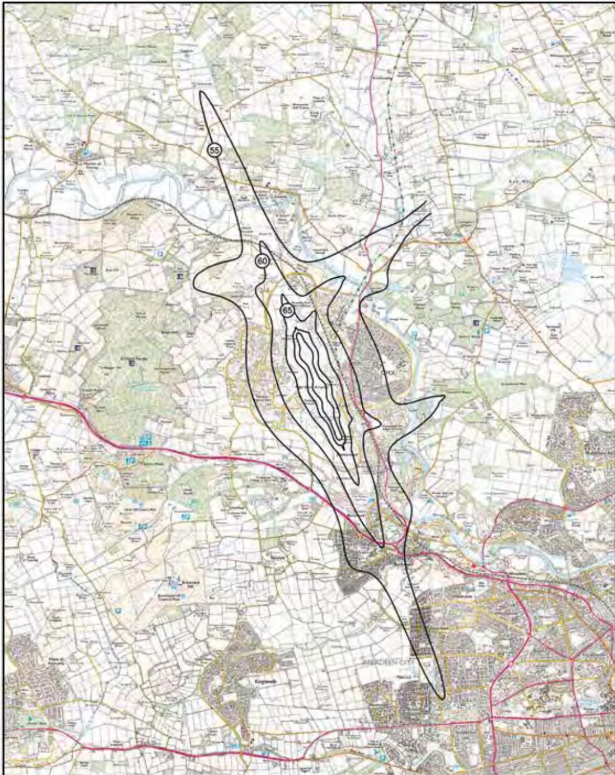
ABERDEEN INTERNATIONAL AIRPORT 2016 Annual Day L_{Aeq,16hr} 55-75 dB(A) Noise Contours (Fixed-Wing + Helicopters) Actual Modal Splits: Fixed-Wing 52% S / 48% N, Helicopters 64% S / 36% N
