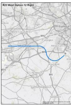
short straight segment before making a left turn to the west, just to the north of Lymm where it combines with the option from 23R. The combined routes continue in a westerly direction routing overhead Warrington and terminate at 7,000ft just north of Widnes.
