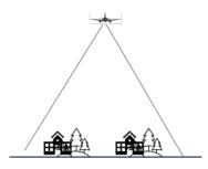
Alternatively, by looking at this from an aircraft's perspective, all buildings and locations within the cone are 'overflown'.
