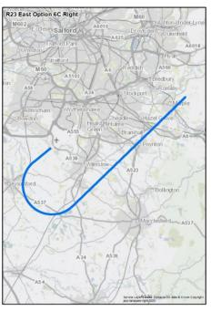
A speed restriction of 190 KIAS is used for the first turn which allows the smallest radius. Although PANS-OPS compliant it should be assessed for flyability as part of the procedure validation process within Stage 4 of CAP1616.
