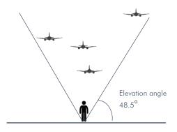
CAP1616 recommends the use of 48.5° as an elevation angle. This is because for an aircraft to give a noise level approximately 3dB lower than if it had flown directly overhead, it would need to be at an elevation angle of 48.5°. 3dB is widely accepted as the smallest difference between two noise levels that the average person can perceive.
