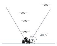
CAP 1616 recommends the use of 48.5° as an elevation angle. This is because for an aircraft to give a noise level approximately 3dB lower than if it had flown directly overhead, it would need to be at an elevation angle of 48.5°. 3dB is widely accepted as the smallest difference between two noise levels that the average person can perceive.
