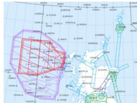
Figure 8: Option 4 – Example of what a new bespoke airspace design might look like
