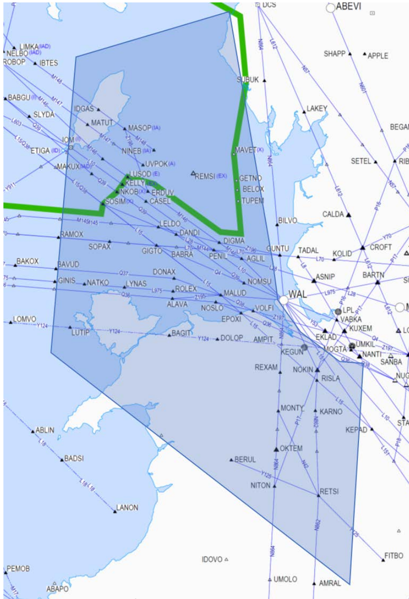
Figure 34: Adapted internal airspace map showing the lower airspace routes contained within the lateral limits of the Western Arm (blue polygon).
