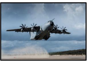
Atlas C.1 (A400m) provides airlift and strategic oversized lift capabilities complementing those of the Hercules and C-17 fleets. It can accommodate as many as 116 fully equipped troops or a combination of vehicles, pallets, and personnel, up to a payload of 37 tonnes. Loads are delivered by parachute, gravity extraction or by landing. Paratroops will be dropped from the aircraft's dedicated paratroop doors, or from the rear ramp.
