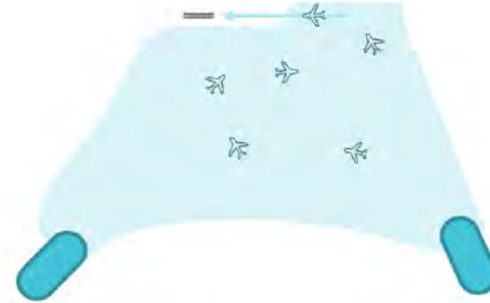
Hold(s) further out - more than 30nm (Linked with either a traditional Radar Manoeuvring Area (RMA) or Transitions)
