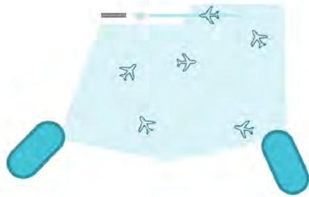
Optimised Hold(s) - within 30nm (Linked with either a traditional Radar Manoeuvring Area (RMA) or Transitions)
