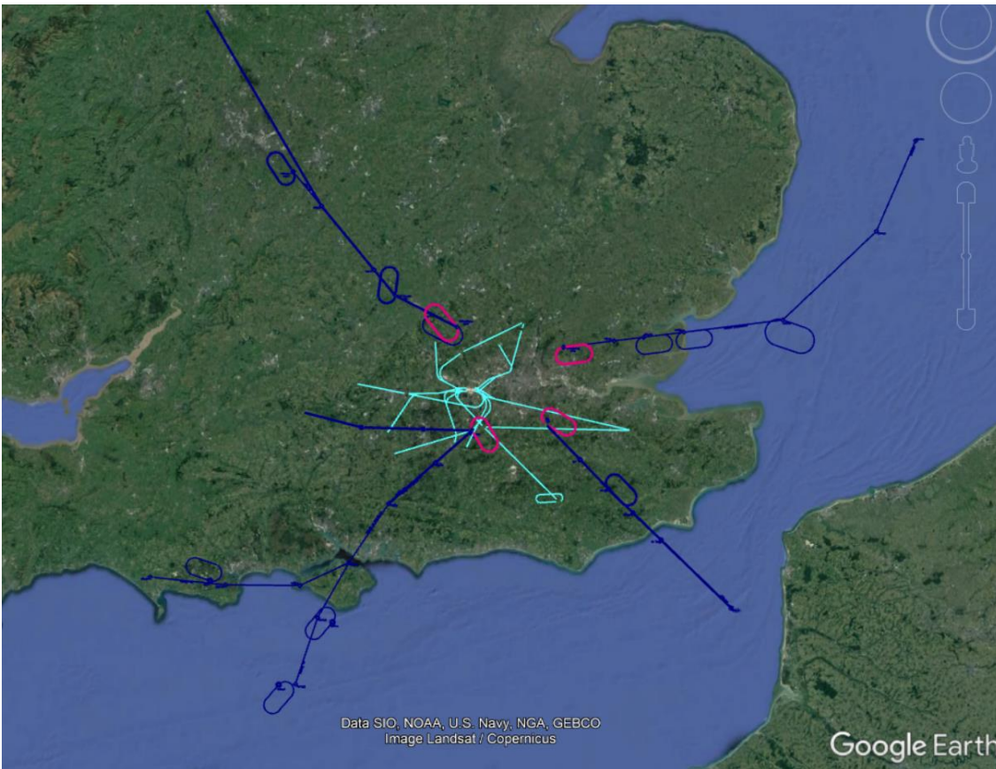
Figure 1 Current arrival and departure procedures for Heathrow
