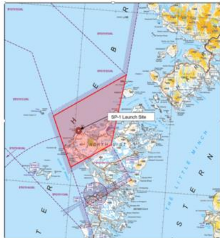
Figure 3: Diagram depicting the original proposed airspace 'fillet' design over SP-1 launch site
