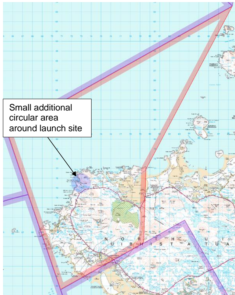
Figure 3: Small circular area of segregated airspace within 'fillet' to protect SP-1 ground personnel
