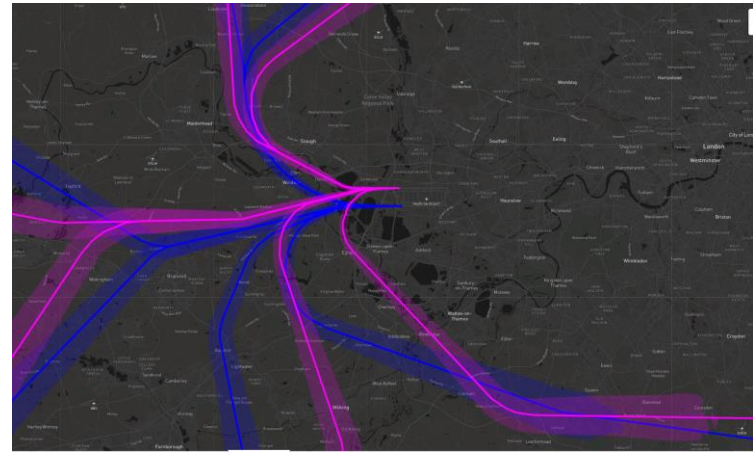
Example of departure routes which are kept apart for longer after departure
