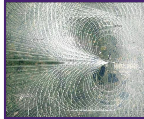
Sample of notional tracks for westerly departures from the northern runway – known as “27R departures”
